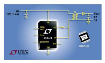
output load current in a typical application. Boundary mode operation also permits the use of a smaller transformer when compared to equivalent continuous conduction mode designs. The output voltage is easily set by two external resistors.
