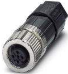
Sensor/actuator connector, socket, straight, 4-pos., M12 SPEEDCON, A-coded, spring-cage connection, metal knurl, cable diameter max. 8 mm
