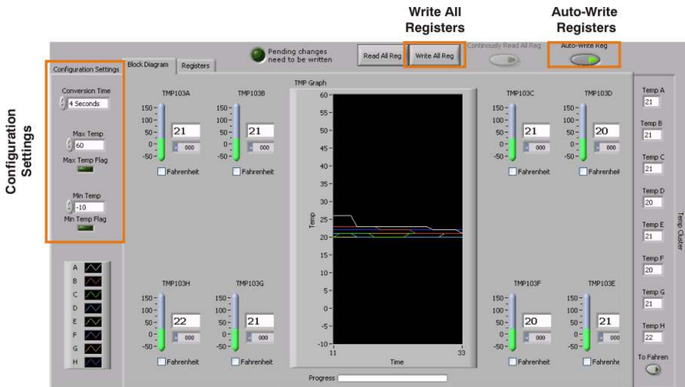
Figure 17. TMP103EVM Software: Writing to Registers
