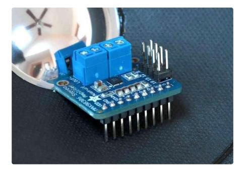
This incredibly small stereo amplifier is surprisingly powerful - able to deliver 2 x 3.7W channels into 3 ohm impedance speakers. Inside the miniature chip is a class D controller, able to run from 2.7V-5.5VDC. Since the amp is a class D, its incredibly efficient (over 90% efficient when driving an  $8\Omega$  speaker at over a Watt).
