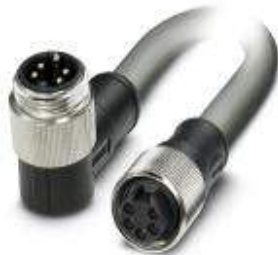
Bus system cable, DeviceNet, 5-position, PVC, Gray RAL 7001, Plug angled 7/8"-16UNF, on Socket straight 7/8"-16UNF, Cable length: 10 m
