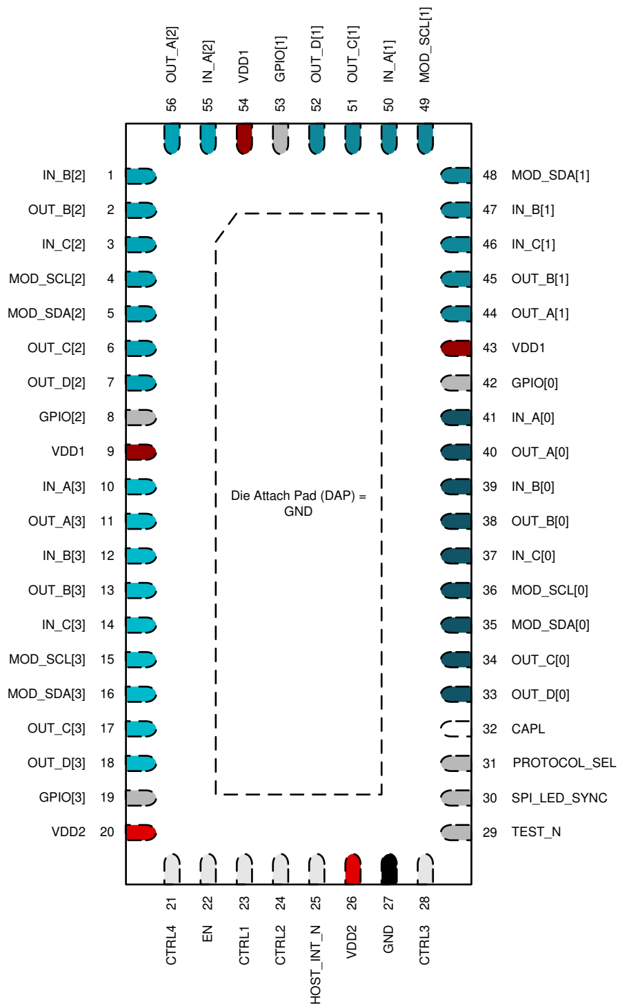
Figure 6-1. RHU Package 56-Pin WQFN Top View
