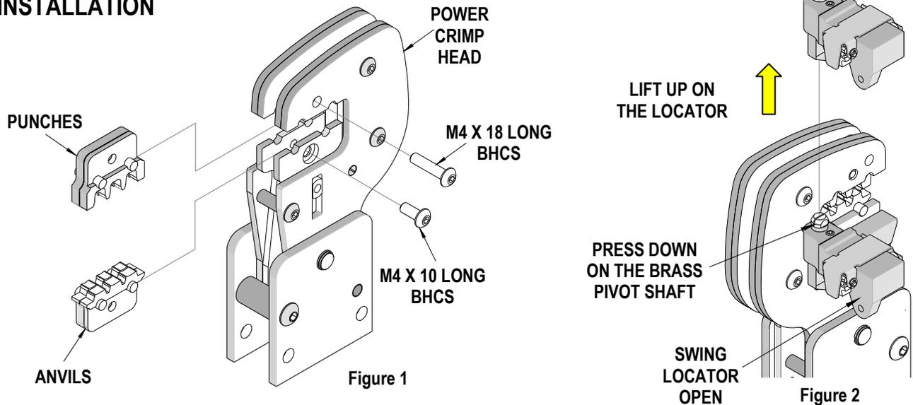
To install the Tool Kit into the Power Crimp Head follow the steps below:
