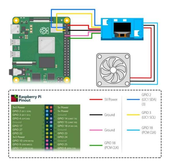
NOTE: The RGB lights in the fan are connected to the ambient lights on the screen driver board. Turn on any one of the lights is equivalent to turn on the entire light group.
