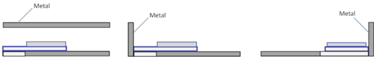
Fig 5-4. Not recommended location in Z plane
