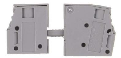
Feed-through terminal, Screw connection, Mounting type: Mounting surface, Rated cross-section: 4 mm<sup>2</sup>, Colour: Grey
