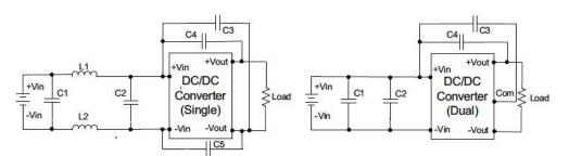
Input filter components (C1 $\sim$ C5, L1/L2) are used to help meet conducted emissions.
