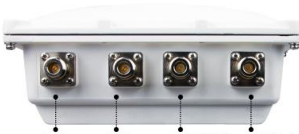
LoRa Antenna Port WiFi Antenna Port LTE-DIV / LoRa2 Antenna Port LTE-Main Antenna Port
