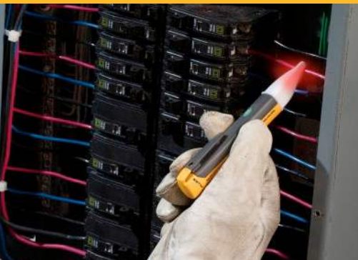
1AC-II with beeper, on-off and self test
