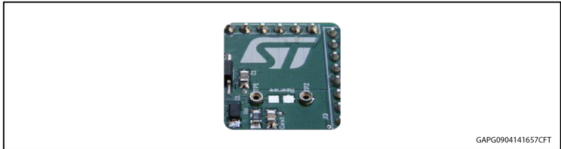
Figure 4: Mounting through-hole sense resistor
