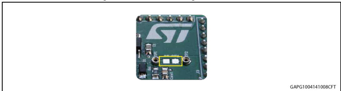
Figure 5: Pads for soldering SMD resistor
