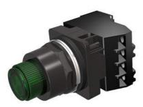
30mm BlackMax, Epoxy Coated Corrosion Resistant Complete Metal Unit PTT / Illuminated Pushbutton Full Voltage, 12V AC/DC Incandescent Lamp Extended Button Plastic Lens, Green 2 Position Momentary with 1 N.O. - 1 N.C. Heavy Duty Contacts, A600/P600 UL Listed, CSA Certified NEMA 1,3,3R,4,4X,12,13 & Automotive Standards
