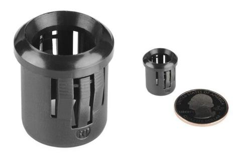
**Description:** These plastic LED holders have a black finish and only need the LED and the holder to be snapped into place easily and effectively, no screwing anything into place. These LED holders accept a 10mm LED and mount into an 35/64" diameter hole.
