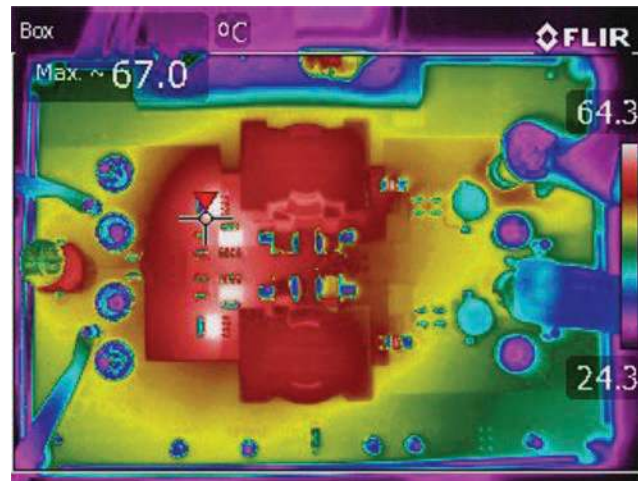
Figure 6. Thermal Map, V_{IN} 48V, V_O 12V, I_O 25A, No Air Flow
