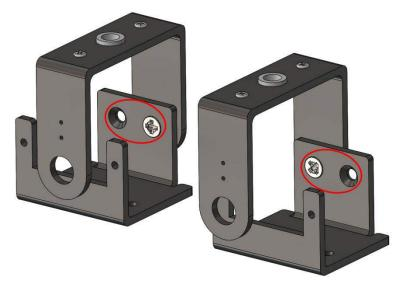
Use two M1.5\*5 self-tapping screws to secure the 1-arm rocker arm on the No.4 board.
