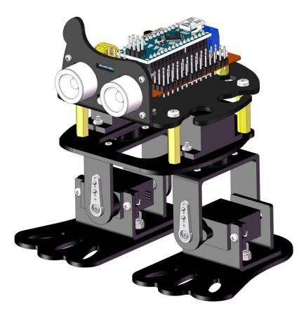
Secure the 2 legs with the smallest screws in the packaged with servo.
