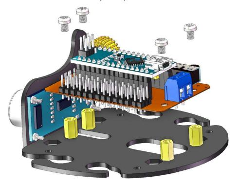
Use M3\*5 screws to fix M3\*25 Bi-pass Copper Standoff under the No. 1 board.
