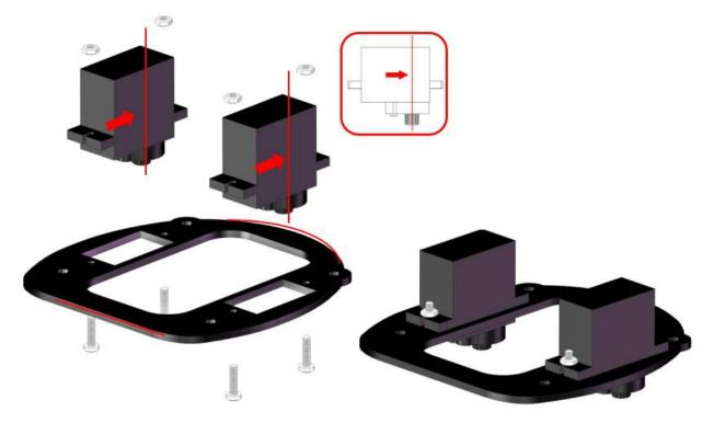
Secure the No. 1 and No. 2 boards with M3\*5 screws. Note that the side of the servo shaft should be mounted on the side of the USB port.
