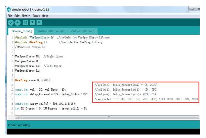
change the value of vel and delay\_Forward in line12 and 13 to as shown:
