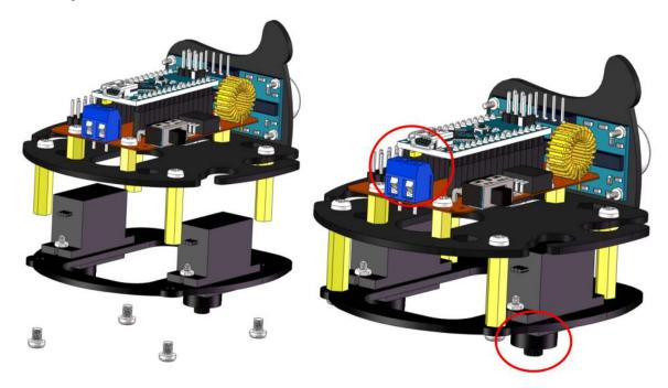
Use two M1.5\*5 self-tapping screws to fix the 2-arm rocker arm to the No. 4 board and use the same method to install another No. 4 board.
