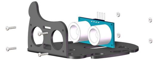
Use a M3\*5 screw to secure the M3\*8 Bi-pass Copper Standoff post on No. 1 board.
