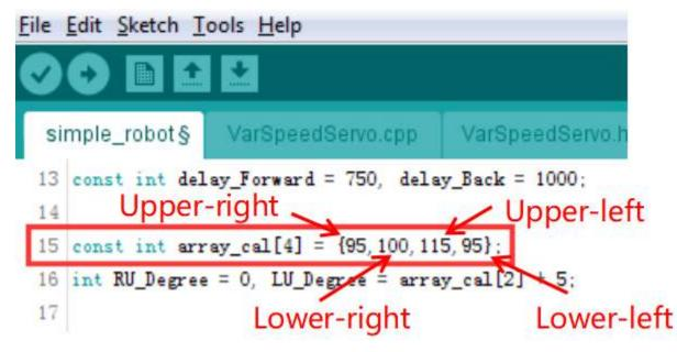
The basic principle of calibration: increased values can rotate the servo shaft clockwise and vice versa. For example, if the right leg is toe out, you need to decrease the upper-right servo's angle; if it is toe in, you need to increase the angle.
