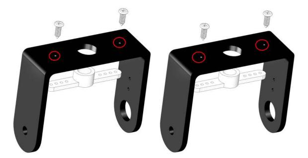
Secure one of the round holes on the 4th and 5th boards with M3\*8 Countersunk screws and M3 self-locking nuts.
