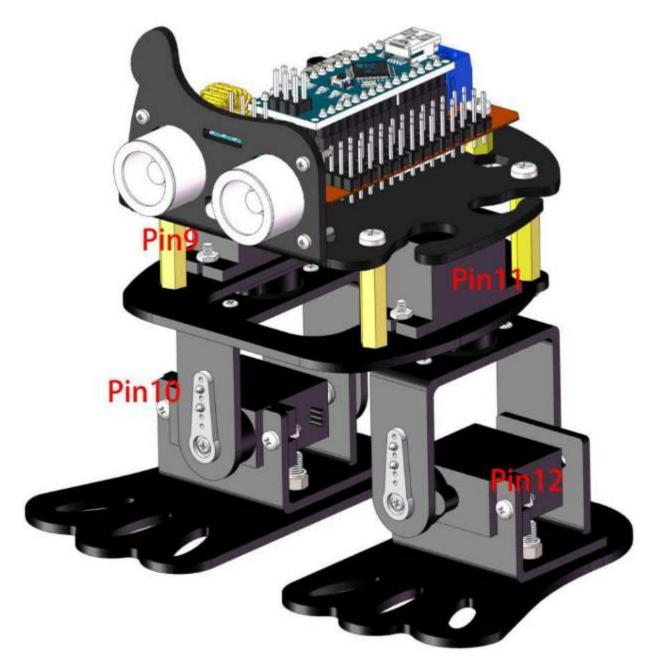
Open the program simple\_robot.ino and go to Line 39. Set #define CALIBRATION as able and disable the other two. Then select the correct board and port, and upload the sketch.
