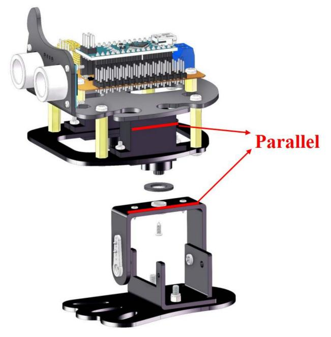
Insert a servo (in working condition) into the servo shaft of the left foot. Besides 2 M2\*8 screws and 2 M2 nuts, a gasket plate is needed between the servo and left leg.
