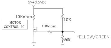
14-1. THE FAN SPEED WILL DEFAULT TO MAXIMUM WHEN THE SPEED CONTROL INPUT IS LEFT UNCONNECTED.
