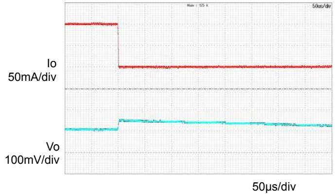
Figure 9. Transient Response ( T_a=25^\circ\text{C} ) ( I_o = 0.1\text{A}\rightarrow 0\text{A} )
