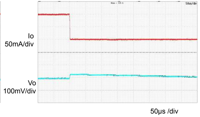
Figure 11. Transient Response ( T_a=-40^\circ\text{C} ) ( I_o = 0.1\text{A} \rightarrow 0\text{A} )
