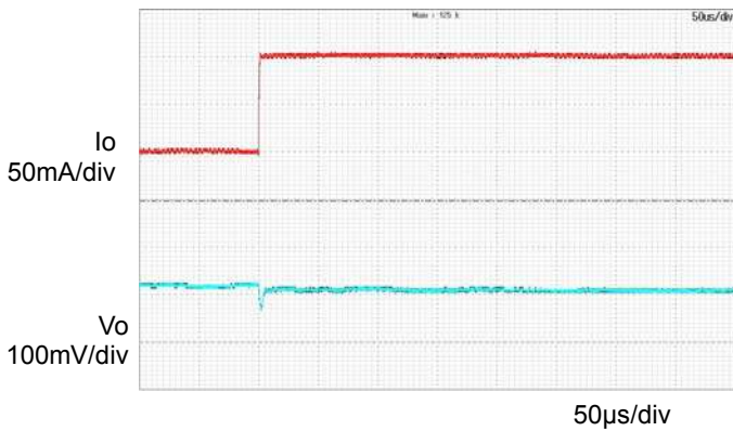
Figure 8. Transient Response ( T_a=25^\circ\text{C} ) ( I_o = 0\text{A}\rightarrow 0.1\text{A} )
