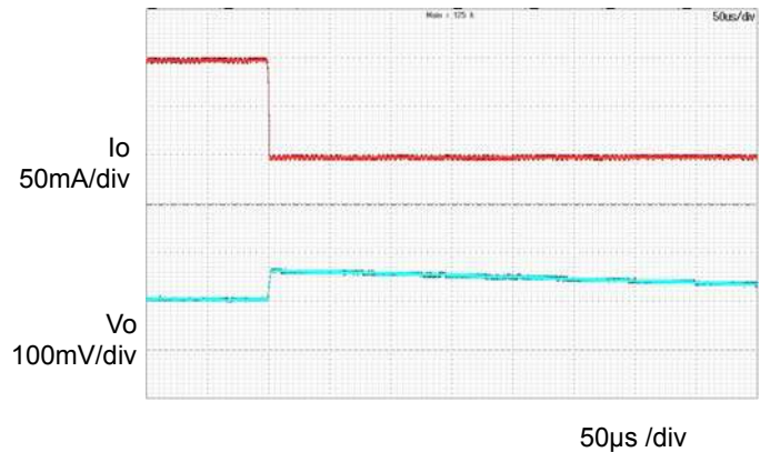
Figure 13. Transient Response ( T_a=105^\circ\text{C} ) ( I_o = 0.1\text{A} \rightarrow 0\text{A} )
