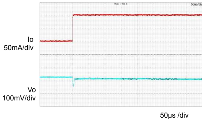
Figure 12. Transient Response ( T_a=105^\circ\text{C} ) ( I_o = 0\text{A} \rightarrow 0.1\text{A} )
