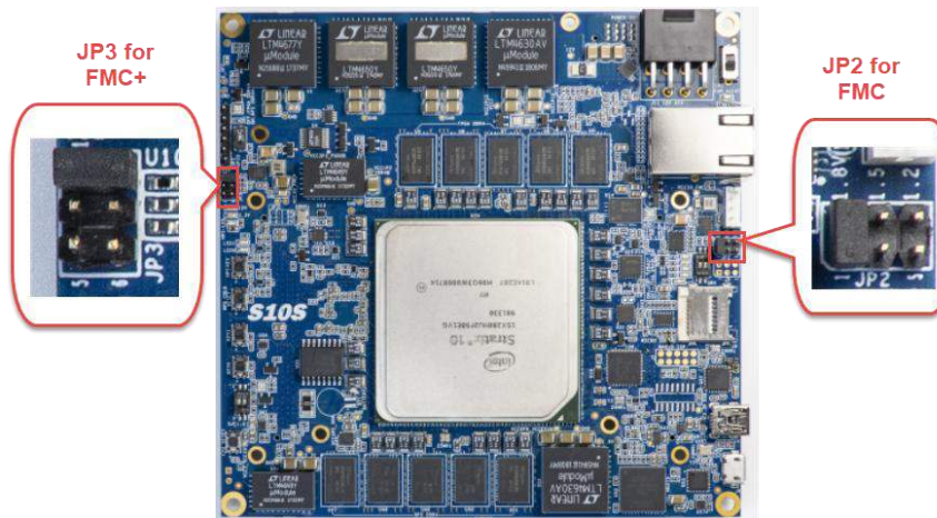
Figure 2-6 FMC and FMC+ I/O standard setting headers
