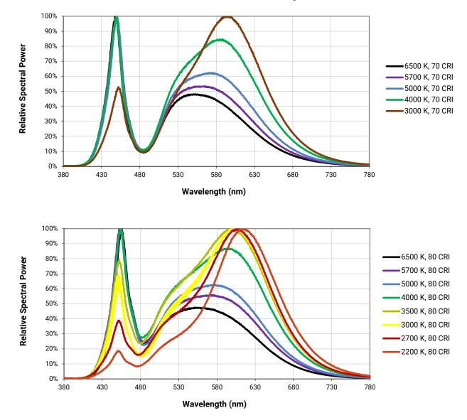
The following graphs are the result of a series of pulsed measurements at 450 mA and  $T_1$  = 85 °C.
