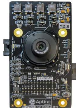
Figure 1. MT9P004 Evaluation Board
