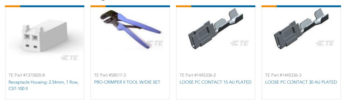
Housing, Receptacle, Wire-to-Wire, 2 Position, .1 in [2.54 mm] Centerline, Crimp, 1 Row, Natural, Mating Retention, Wire & Cable, Power & Signal
