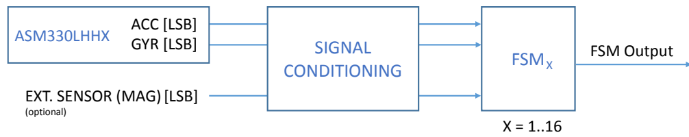
Figure 2. State machine in the ASM330LHHX
