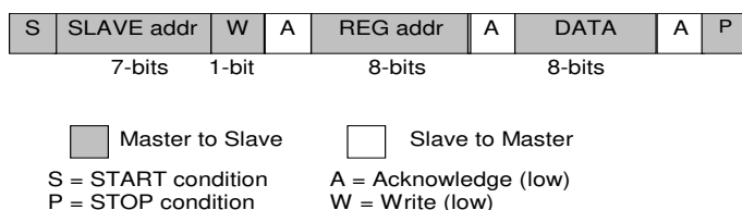
Figure 27: I 2 C byte write (SDA signal)
