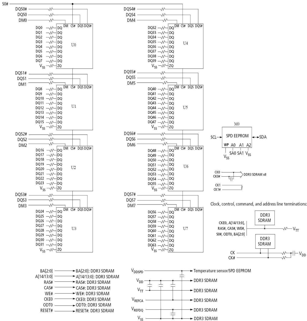
Note: 1. The ZQ ball on each DDR3 component is connected to an external  $240\Omega \pm 1\%$  resistor that is tied to ground. It is used for the calibration of the component's ODT and output driver.
