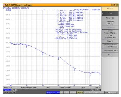
156.25 MHz LVPECL output Phase Noise: 624 fs (12 kHz-20 MHz)
