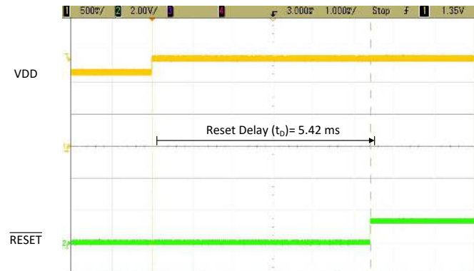
Figure 15. TLV840EVM \overline{\text{RESET}} Delay Time ( t_D ) with C_T Tied to GND Through 0.01- \mu F Capacitor
