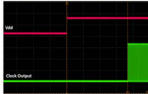
Figure 17. Startup Waveform vs. Vdd
