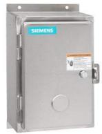
Non-reversing contactor, Size 1 3/4, 4 power poles, Contactor amp rating 40A, 3 wire (NO aux included), 110V 50Hz / 120V 60Hz coil, Non-combination type, Encl NEMA type 4X 304 S-Steel, Water/dust tight noncorrosive, Standard width enclosure
