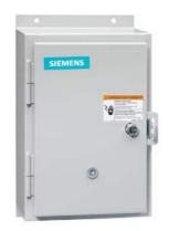
Non-reversing motor starter, Size 1, Three phase full voltage, Solid-state overload relay, OLRelay amp range 5.5-22a, 190 220/220 240V 50/60HZ coil, Non-combination type, Enclosure type 12, Dust/drip proof for indoors, Extra-wide enclosure
