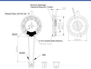
General tolerance =  $\pm 0.5$  mm and all measurements in mm unless otherwise noted.
