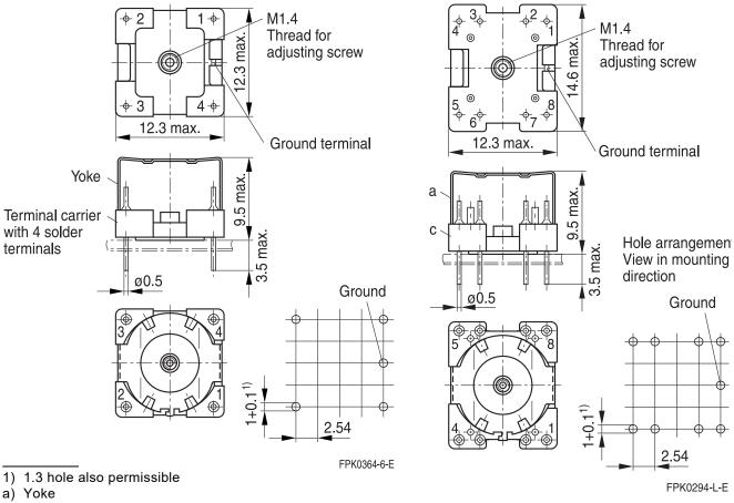
c) Terminal carrier with 8 solder terminals
