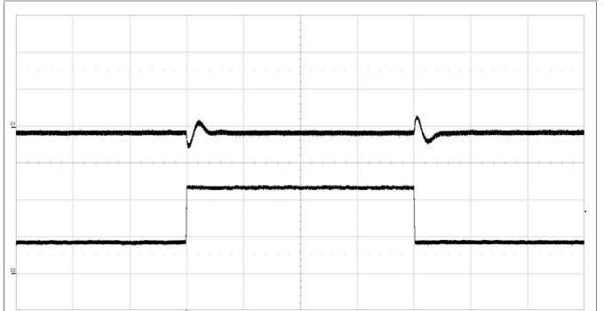
Output voltage response to load current step- change 1.5-4.5-1.5 A at: T_{P1} = +25^\circ\text{C} , V_I = 24\text{ V} . C_{OUT} = 2 \times 47\ \mu\text{F Ceramic} + 330\ \mu\text{F Polymer} Top trace: output voltage 100 mV/div. Bottom trace: load current 2 A/div. Time scale: 100 \mu\text{s} /div. Slew rate: 1A/ \mu\text{s} . 20 MHz bandwidth.
