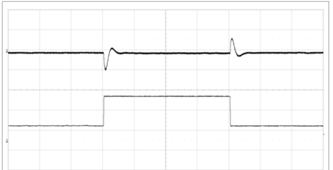
Output voltage response to load current step- change 1.5-4.5-1.5 A at: T_{P1} = +25^\circ\text{C} , V_I = 24\text{ V} . C_{OUT} = 2 \times 47\text{ }\mu\text{F Ceramic} + 330\text{ }\mu\text{F Polymer} Top trace: output voltage 50 mV/div. Bottom trace: load current 2 A/div. Time scale: 200 \mu\text{s} /div. Slew rate: 1A/ \mu\text{s} . 20 MHz bandwidth.
