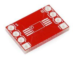
**Description:** 8-Pin SSOP to DIP break out board. The footprint was rotated to accommodate different width SSOP devices and can be used with 8 pin SSOPs. Designed to be used with 0.65mm pitch devices but can also be used with 0.025" pitch devices (comes out to  $\sim$ 0.635mm). We've made these 0.635mm devices fit just fine. Can be used with packages from 0.200" (5mm) up to 0.450" (11.4mm) in width.
