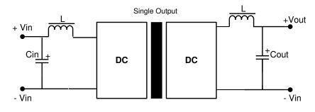
It is not recommended to connect any external capacitor in the application field when output loading is less than 0.5 watt.
