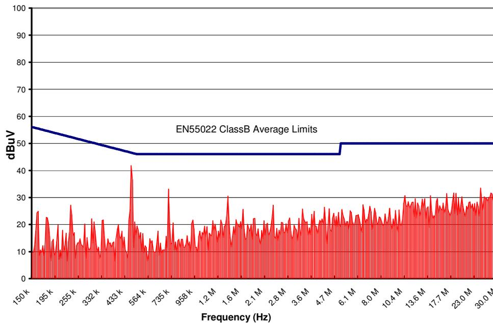
Figure 17. CPT20F48 Conducted Emissions using above specified input filter.
