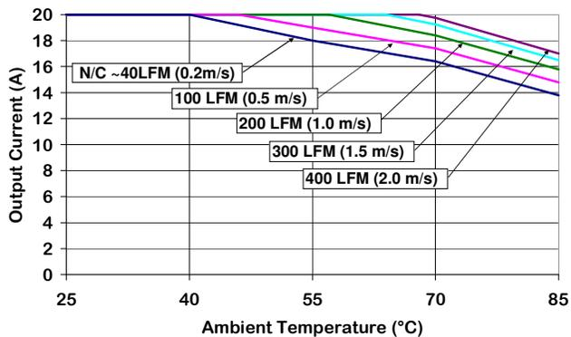
Figure 3. Output Current Derating vs Ambient Temperature & Airflow (converter mounted vertically with air flowing from pin 3 to pin 1, Vin = 48 V.)
