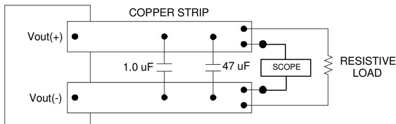
Use a 1.0 $\mu$ F X7R ceramic capacitor and 47 $\mu$ F ceramic capacitor. Scope measurement made using a BNC socket. Position the load 3 in. [76mm] from module.
