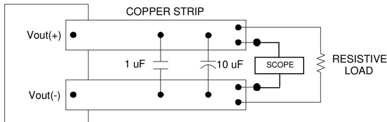
Use a 1 $\mu$ F X7R ceramic capacitor and a 10 $\mu$ F @ 25V tantalum capacitor. Scope measurement should be made using a BNC socket. Position the load 3 in. [76mm] from module.
