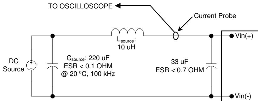
Note: Measure input reflected-ripple current with a simulated source inductance ( $L_{source}$ ) of 10  $\mu$ H. Capacitor  $C_s$  offsets possible source impedance.
