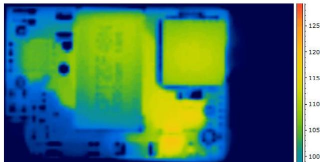
Figure 4. Thermal Image of CPT20F48 (20A output, 55C Ambient, 200lfm airflow, Vin = 48V, airflow from pin 3 to pin 1, T<sub>max</sub> = 120°C)
