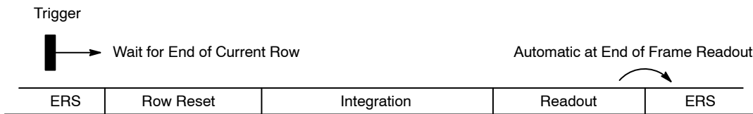
Figure 33. Entering and Leaving a Global Reset Sequence
