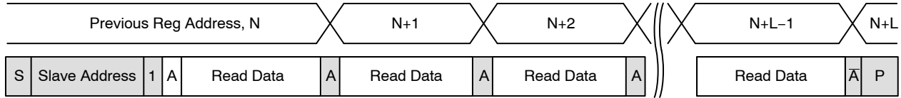
Figure 12. Sequential READ, Start from Current Location
