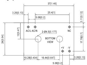
Case No.IRM03 Unit:mm[inch] Tolerance:±0.5[±0.02] unless otherwise specified
