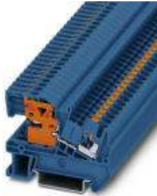
N disconnect terminal block, Push-in connection, Cross section: 0.14 mm 2 - 4 mm 2 , AWG: 26 - 12, Width: 5.2 mm, Color: blue, Mounting type: NS 35/7,5, NS 35/15
