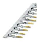
Crimp contact, Pin, rolled, Taped articles, number of pieces per reel: 500, contact diameter: 1 mm, crimp range:  $0.22 \text{ mm}^2 \dots 0.56 \text{ mm}^2$ , Item is lead-free in accordance with RoHS II without Exemption 6c (Pb <0.1%)
