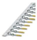
Crimp contact, Pin, rolled, Taped articles, number of pieces per reel: 10000, contact diameter: 1 mm, crimp range: 0.08  $\rm mm^2$  ... 0.22  $\rm mm^2$
