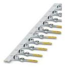
Crimp contact, Pin, rolled, Taped articles, number of pieces per reel: 10000, contact diameter: 1 mm, crimp range: 0.22 mm<sup>2</sup> ... 0.56 mm<sup>2</sup>, Item is lead-free in accordance with RoHS II without Exemption 6c (Pb <0.1%)
