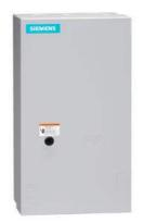
Non-reversing contactor, Size 3 1/2, Three phase full voltage, Contactor amp rating 115A, 3 wire (NO aux included), 380-440/440-480V 50/60Hz coil, Non-combination type, Enclosure NEMA type 1, Indoor general purpose use, Extra-wide enclosure
