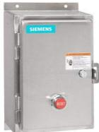
Non-reversing motor starter Size 1 Three phase full voltage Solid-state overload relay OLRelay amp range 3-12A 190-220/220-240V 50/60HZ coil Combination type Water/dust tight non-corrosive
