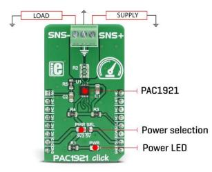
PAC1921 IC is able to integrate the measurements so that the average value can be calculated. The integration can be done in two modes: Free-Run mode and Pin Controlled mode.
