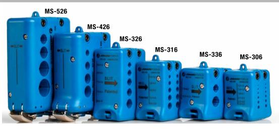
These PATENTED slit and ring tools are designed to open fiber jackets and loose buffer tubes to provide easy fiber access. One side of the tool slits fiber jackets and loose buffer tubes, the opposite side rings fiber jackets and loose buffer tubes. All this is done without damage to the fiber. Blades are replaceable. Note: MS-326 is designed for cables used in ducts and microducts.
