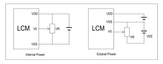
VDD-V0: LCD Driving Voltage
