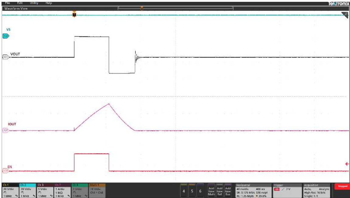
Figure 9-13. TPS281C30 Inductive Discharge (400 mH)
