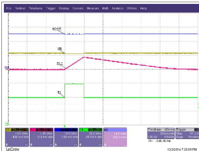
Figure 54. 60A Load Step for 200 ms
