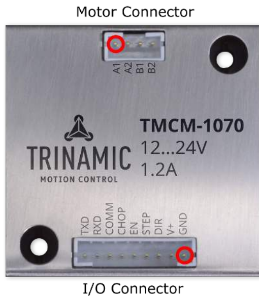
Figure 9: PD42-1070 connectors (pin 1 highlighted in red)
